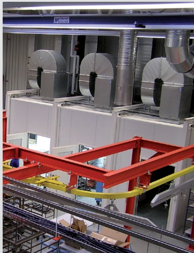
Kleinteile-Lackierkabine 2,5m x 3,5m x 2,8m Paint spraying cabins for small parts, 2,5m x 3,5m x 2,8m
